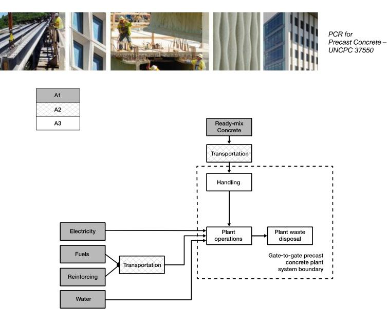
Cradle-to-gate precast concrete plant system boundary
